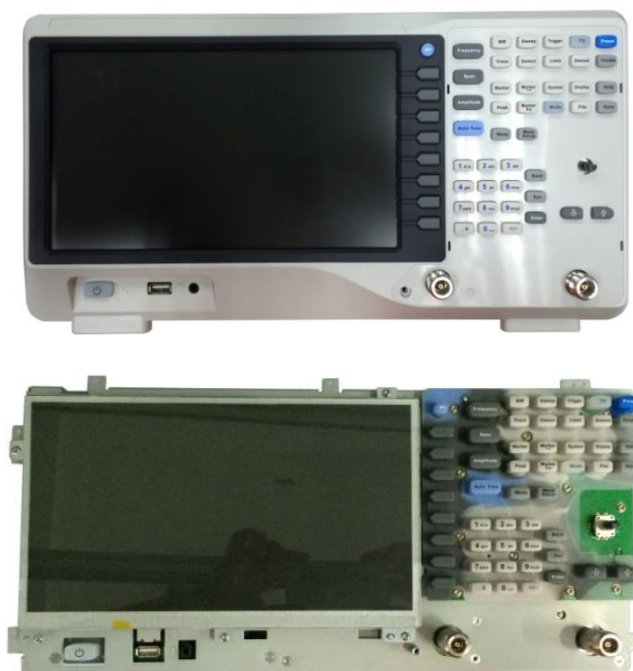
Figure 4-2 Removing the front panel
