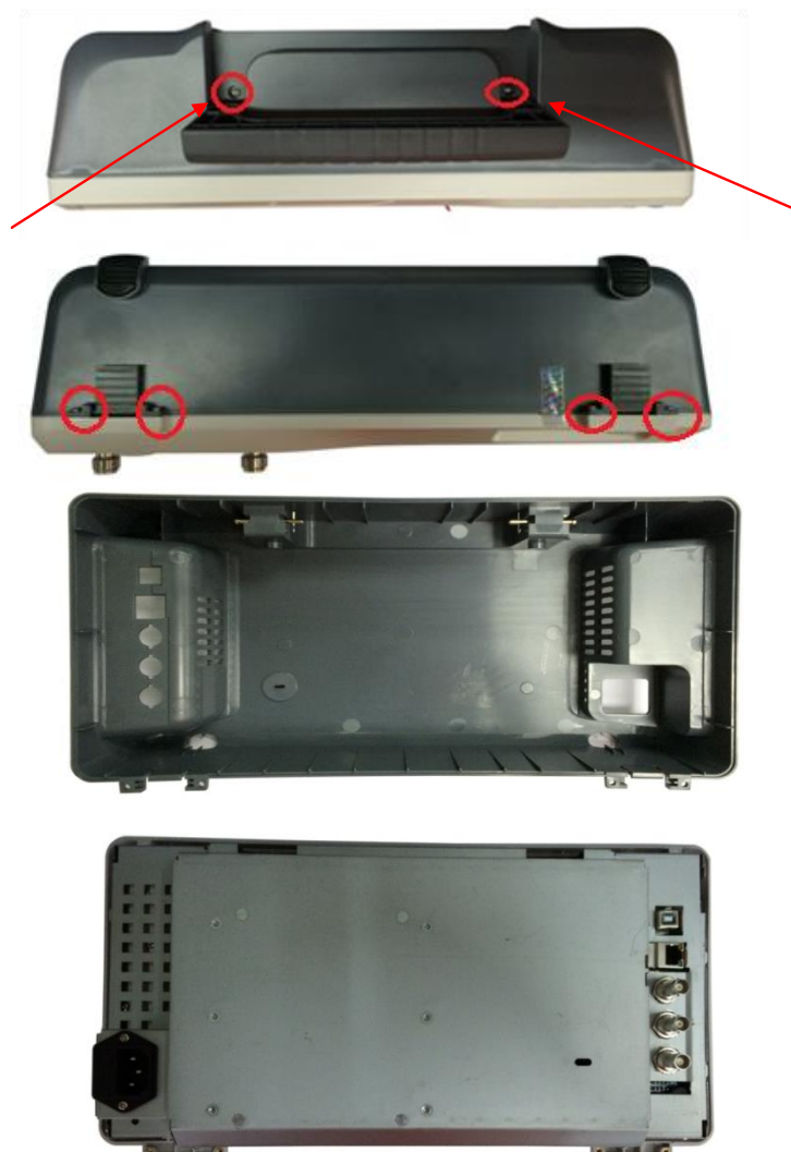
Figure 4-1 Removing the Rear Panel Screws
